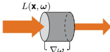
$$(\omega \nabla) L(\mathbf{x}, \omega) = \underbrace{-\sigma_t(\mathbf{x}) L(\mathbf{x}, \omega)}_{Extinction} + \underbrace{\sigma_s(\mathbf{x}) L_s(\mathbf{x}, \omega)}_{In-scattering} + \underbrace{\sigma_a(\mathbf{x}) L_e(\mathbf{x}, \omega)}_{Emission} \quad (2)$$
