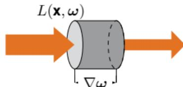
$$(\omega \nabla) L(x, \omega) = \underbrace{-\sigma_t(x)L(x, \omega)}_{Extinction} + \underbrace{\sigma_s(x)L_s(x, \omega)}_{In-scattering} + \underbrace{\sigma_a(x)L_e(x, \omega)}_{Emission} \quad (1)$$
